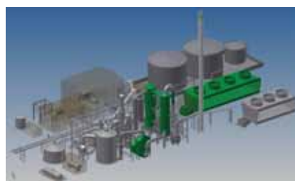
Acid plant makeover: green shows some of the extent of the upgrade. The absorbing towers were made from Saramet, a new corrosive-resistant material.
