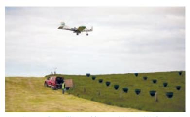
Ravensdown's IntelliSpread $^{\text{TM}}$  system delivers a variable rate of fertiliser via the computer-controlled automatically adjusting hopper doors. In late 2015, researchers tested the modelled predictions compared to where fertiliser actually lands. The results were positive.
