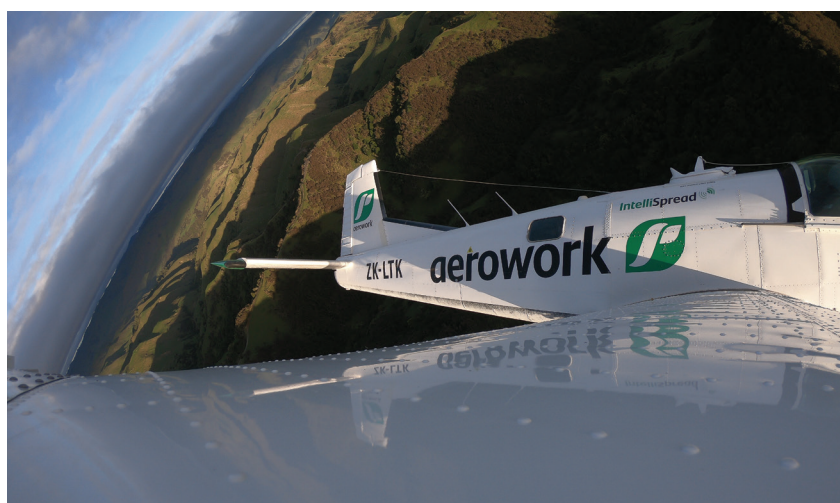
A soil fertility map directs GPS-enabled topdressing aircraft to deliver fertiliser where needed
