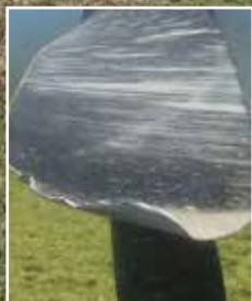
RESULTS OF PROPELLER STRIKE
