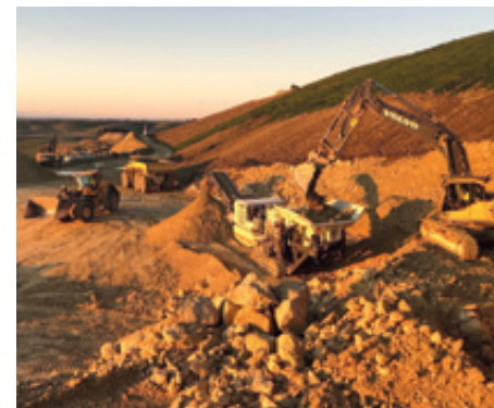
Geraldine primary crusher was replaced to meet increased demand at lower cost and with reduced fuel use and emissions.
