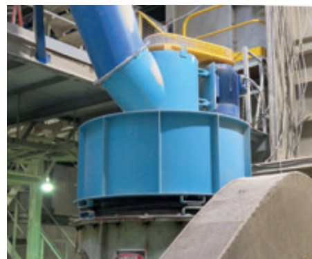
Dunedin dynamic separator improved processing capability while reducing operational and maintenance costs.
