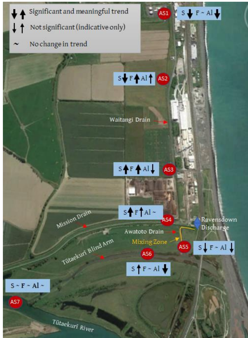
Figure 6. Trends in sulphur, fluoride and aluminium concentrations under ambient conditions at sites upstream and downstream of the Ravensdown discharge point.
