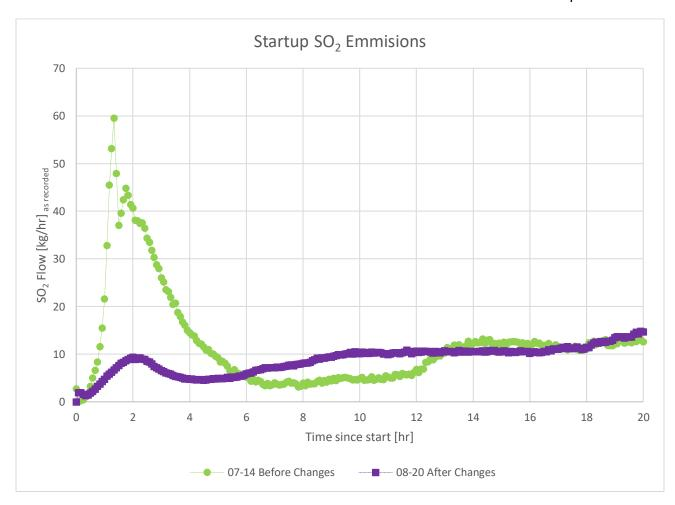
Figure 2: SO<sub>2</sub> emissions during start-ups
